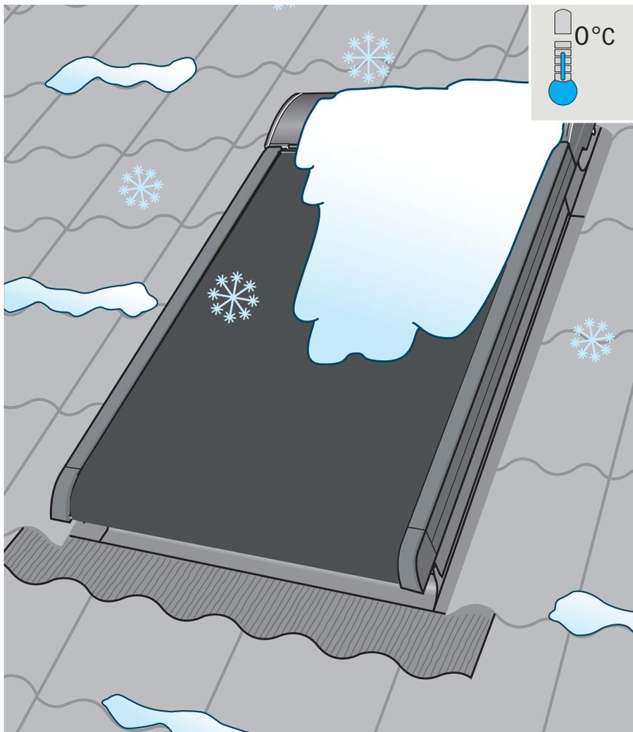
**ENGLISH:** As a precondition to avoiding any damage to the awning blind in very cold regions and in regions with heavy snowfall, either a snow stop or snow-wedge must be installed above the awning blind [a](#), [b](#).
