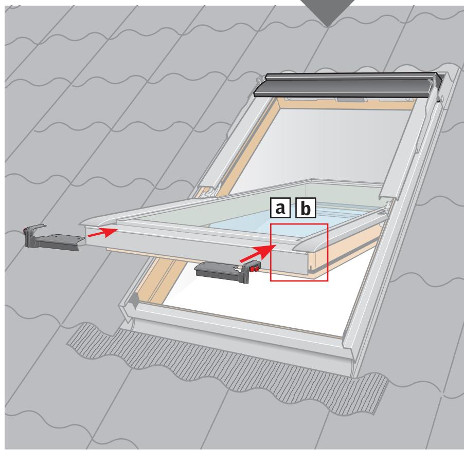
**ENGLISH:** Position bottom brackets temporarily on bottom sash and drill holes for screws. Remove brackets and place sealant on screw holes **a**. Position bottom brackets and fit with screws supplied. Remove transit device **b**.
