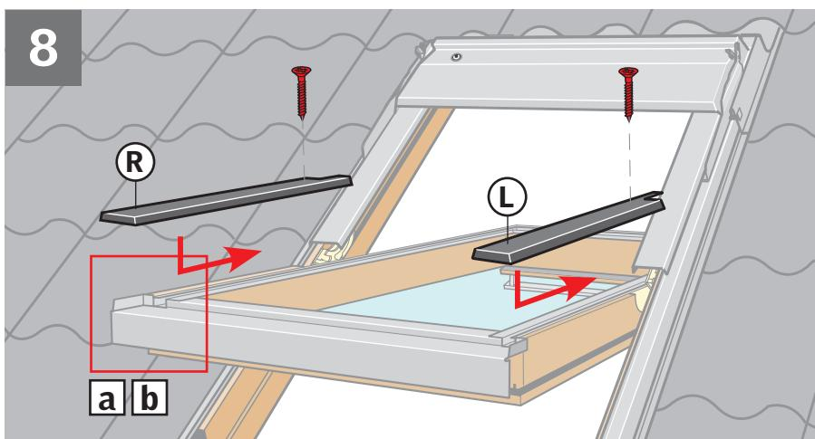
**ENGLISH:** Refit the covers **a**, then drill hole, in sash, through the covers using a Ø 3 mm drill **b**.
