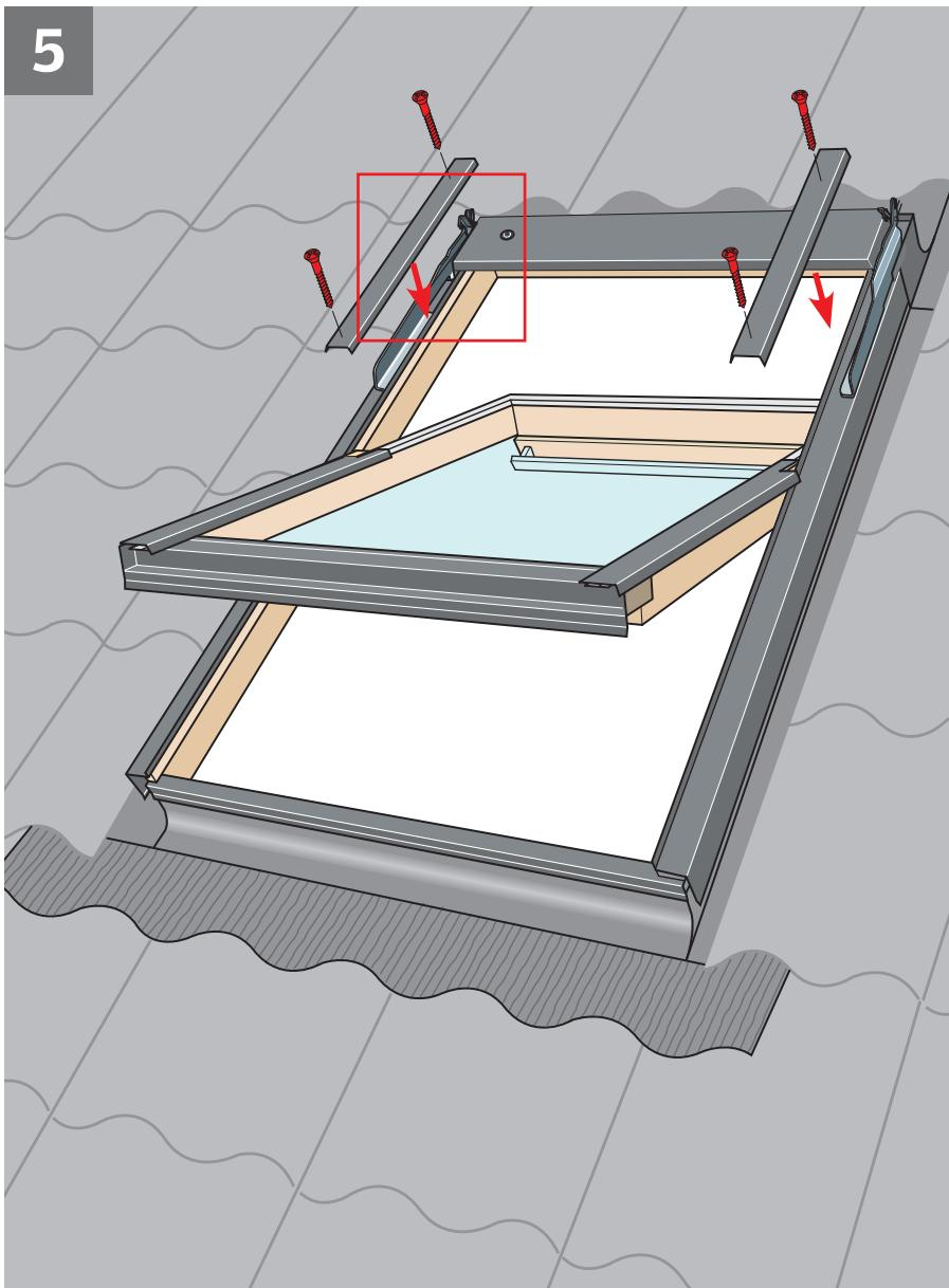
**ENGLISH:** Loosen screws in top cover **a** or **b**. Fit window covers using existing screws. Re-tighten top cover screws.
