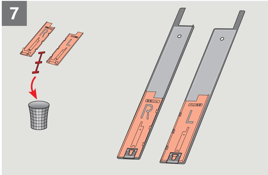
**ENGLISH:** Fit distance sheets (**R** and **L**) on the underside of the covers. Slide the sheets completely down into the cover brackets **a**. Drill holes, through the covers, at the marks using a Ø 5 mm drill **b**.
