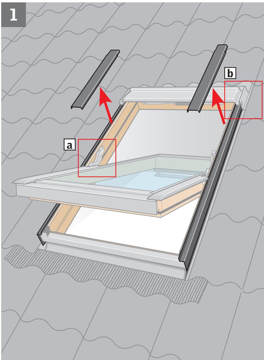
**ENGLISH:** Remove covers indicated temporarily by releasing the snap locks **a**. Drill hole through the mark at the top of the side frame covers. Place sealant on **all** screw holes **b**.
