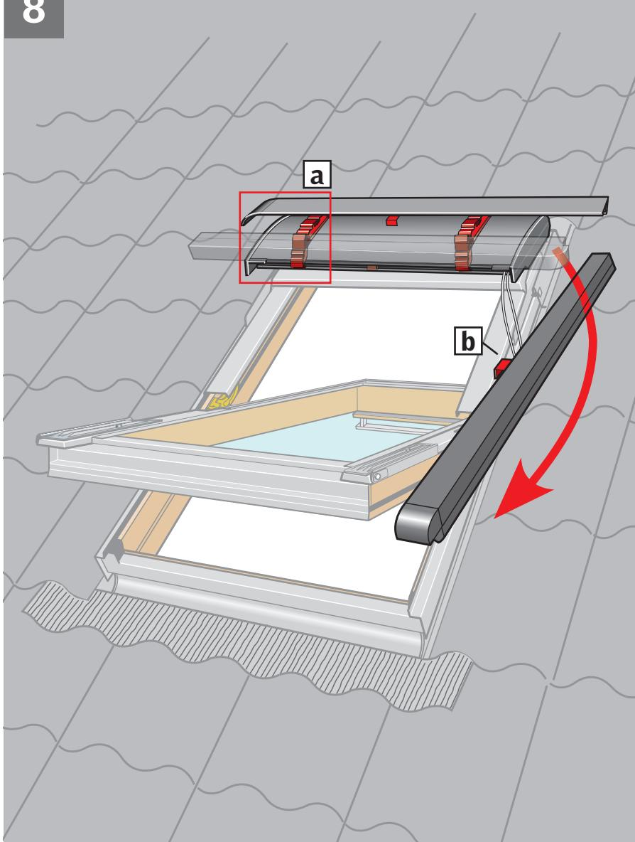
**ENGLISH:** Disengage the first side channel from the transit brackets **a**, turn and hold parallel to side frame. Do **not** remove the transit device **b** at this stage.
