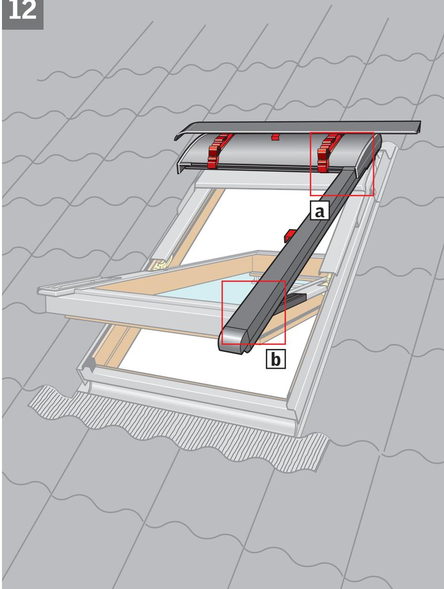
**ENGLISH:** Pull side channel downwards. **It is necessary to pull the side channel hard.** Lift the awning top cover and slide the side channel straight into the groove in the top cover. Ensure that the cords do not cross each other and that they are positioned in the side channel **a**. Snap sliding device **c** onto the bottom bracket **b**.
