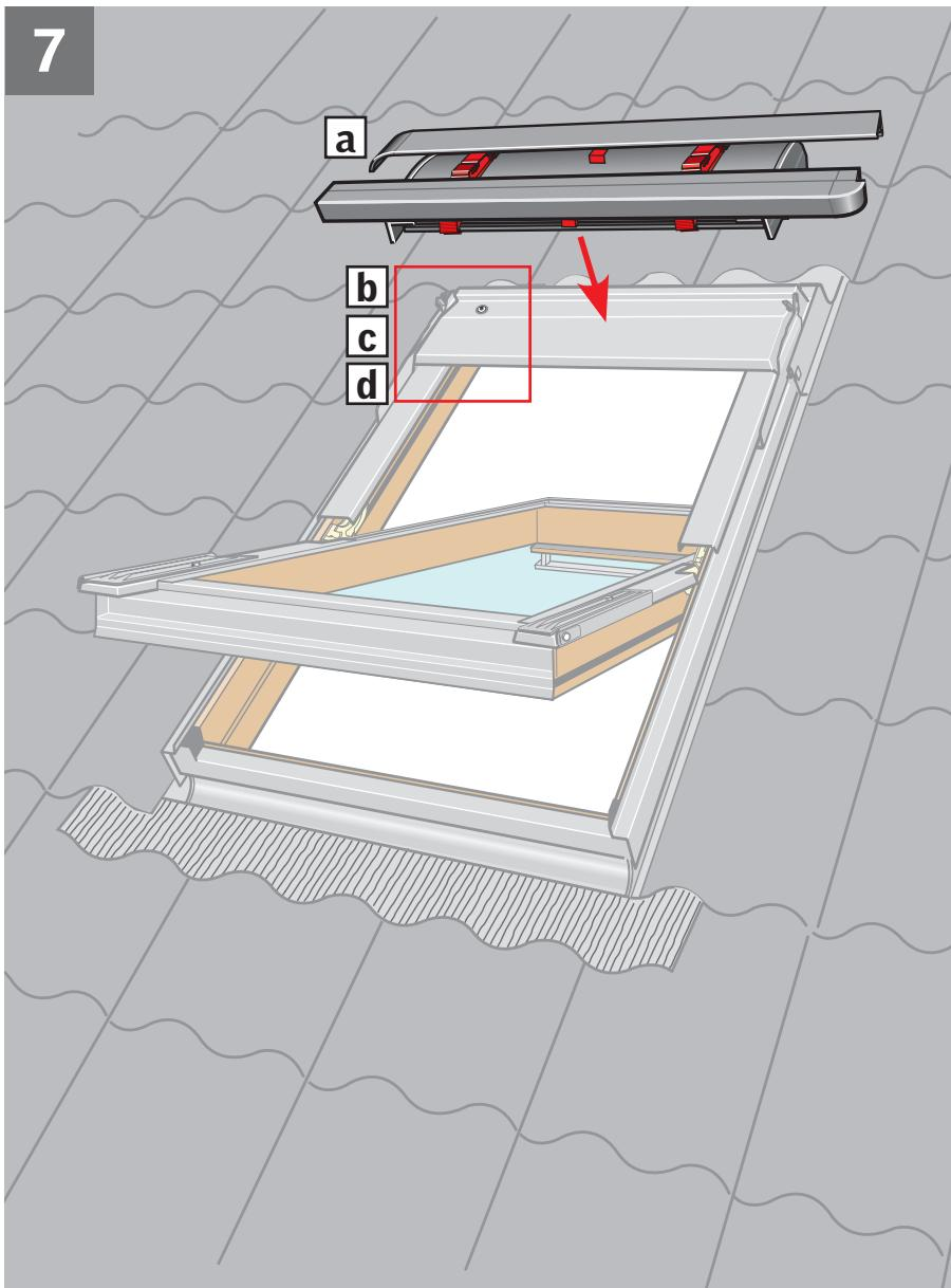
**ENGLISH:** Position awning blind **a**. Fit the awning blind into the bracket and lock it in place **b**. Pull wire through grommet **c**. Ensure that the locking bracket is pressed fully home **d**.
