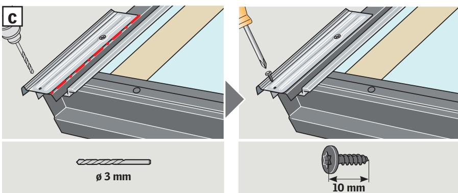
**ENGLISH:** Remove and discard cover screws **a**. Place sealant on screw holes. Fix bottom brackets with 45 mm screws supplied **b** and adjust so that they are parallel to the cover. Drill hole in cover through hole in bracket and fix bracket with 10 mm screw supplied **c**.
