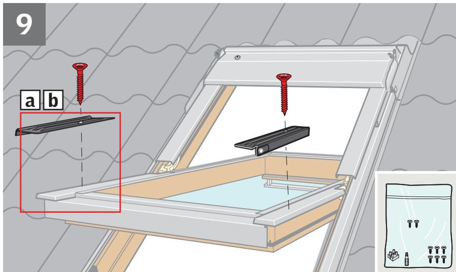
**ENGLISH:** Place sealant on screw holes **a**. Fit bottom brackets with screws supplied **b**.
