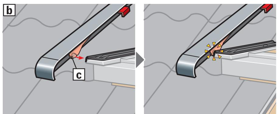
**ENGLISH:** Pull side channel downwards. **It is necessary to pull the side channel hard.** Lift the awning top cover and slide the side channel straight into the groove in the top cover. Ensure that the cords do not cross each other and that they are positioned in the side channel **a**. Snap sliding device **c** onto the bottom bracket **b**.
