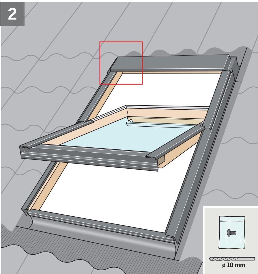
**ENGLISH:** If the window has been fitted with a connection box, remove this temporarily **a**. Position of hole depends on the width **X** of the top cover. Determine the width and drill hole **b**. Fit rubber grommet. Pull grommet through from the inside **c**.
