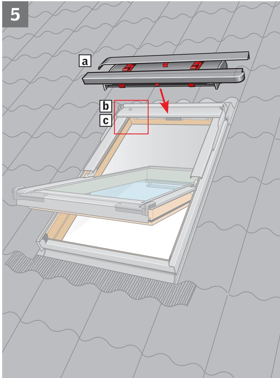
**ENGLISH:** Position awning blind **a**. Fit the awning blind into the bracket and lock it in place **b**. Ensure that the locking bracket is pressed fully home **c**.
