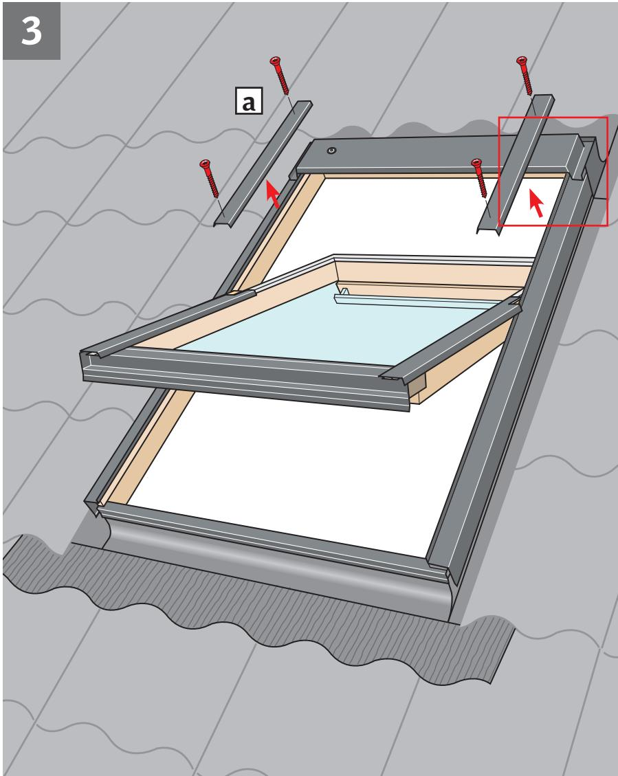
**ENGLISH:** Remove covers indicated temporarily **a**. If there is a screw, remove it **b**. If there is a mark at the top instead of a screw, drill hole through mark **c**. If there is neither screw nor hole, measure position of hole. The position of the hole depends on whether the side frame cover has an upturned edge or not **d**, **e**. If **d** or **e** has been chosen, subsequently drill hole as shown in **c**.
