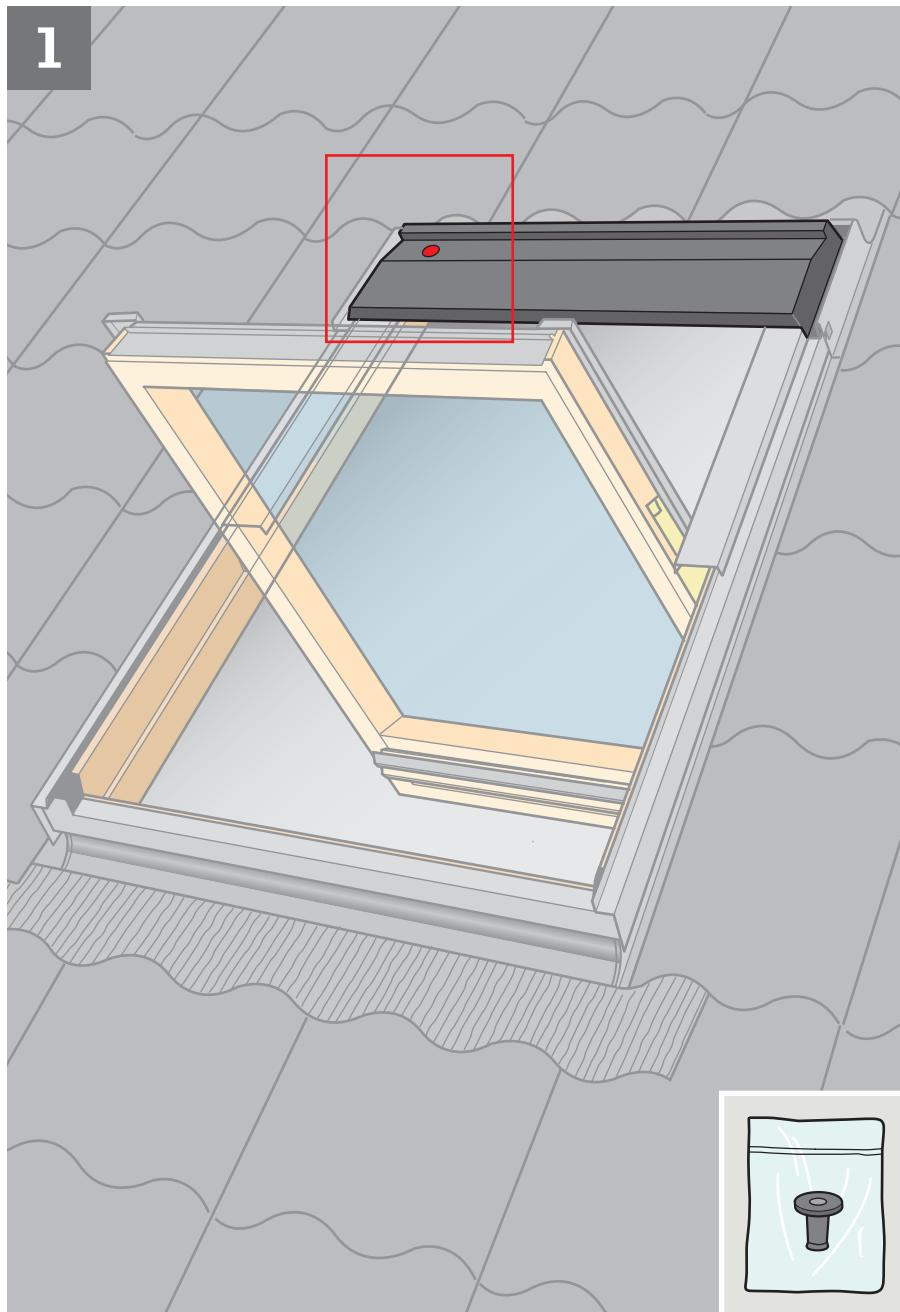
**ENGLISH:** If the window has been fitted with a black screen profile, remove this temporarily **a**. For VELUX INTEGRA® roof windows GGL/GGU, remove the connection box temporarily **b**. Drill hole **c**, and fit rubber grommet **d**. Pull grommet through from the inside **e**.
