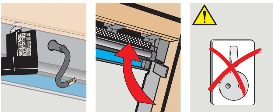
**ENGLISH:** Connect the cable to terminal block or connection box. For connection to control unit, refer to instructions for control unit/remote control. If the window was fitted with a black screen profile and/or a connection box, refit profile/box.
