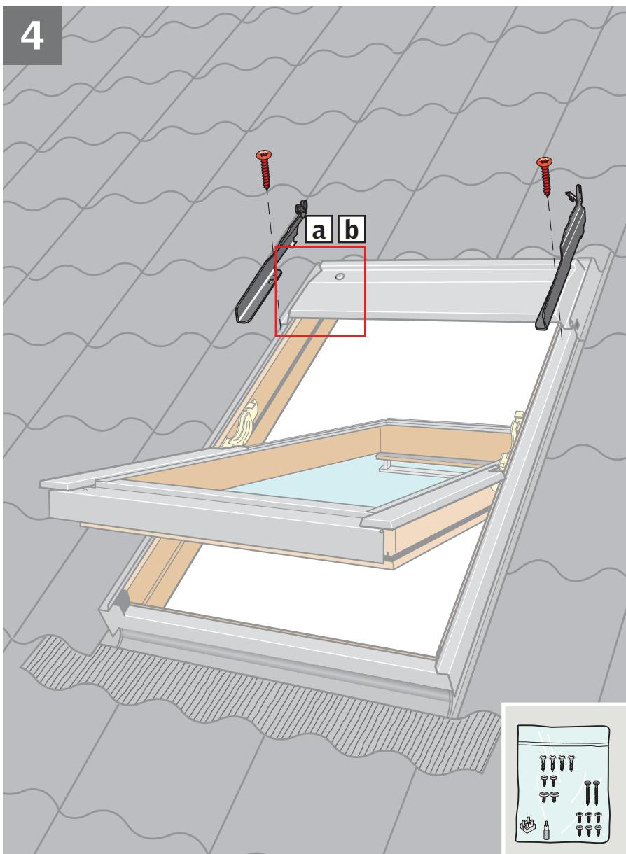
**ENGLISH:** Fix top brackets of awning blind in the round holes with screws supplied. Use 30 mm screw (**GPL/GPU:** 20 mm screw) **a**.
