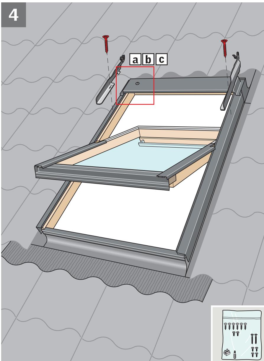
**ENGLISH:** Place sealant on **all** screw holes **[a]**. Fix top brackets of awning blind in slot with screws supplied. Use 30 mm screw (**GPL/GPU**: 11 mm screw) **[b]**. Lift up locking brackets **[c]**.
