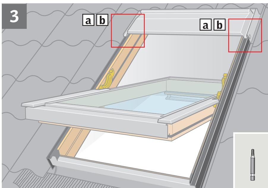
**ENGLISH:** Remove cover screw **a**. If there is a mark at the top instead of a screw, drill hole through mark **b**. Place sealant on **all** screw holes **c**.
