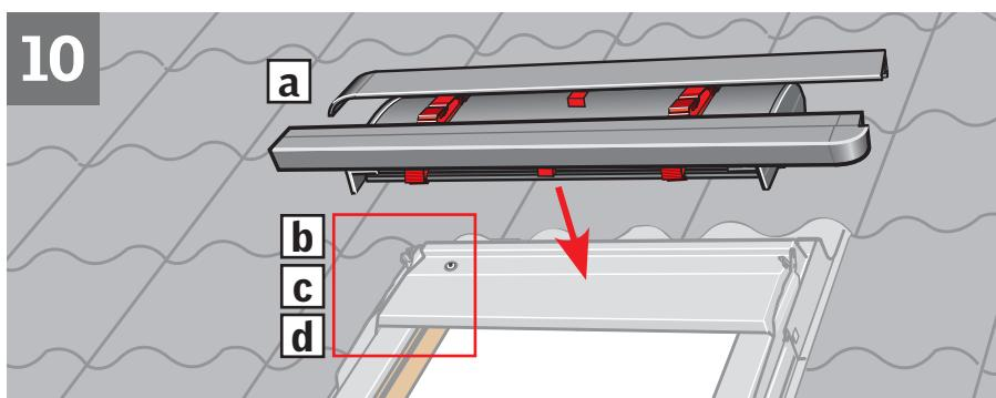
**ENGLISH:** Position awning blind **a**. Fit the awning blind into the bracket and lock it in place **b**. Pull wire through grommet **c**. Ensure that the locking bracket is pressed fully home **d**.
