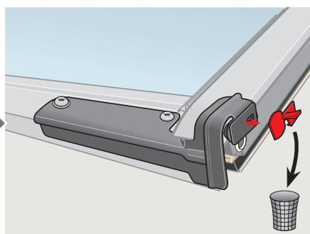
**ENGLISH:** Position bottom brackets temporarily on bottom sash. Drill a pilot hole for screw with a Ø 3 mm drill bit and make a mark with bradawl through the other hole. Remove brackets and place sealant on screw holes **a**. Position bottom brackets and fit with screws supplied. Remove transit device **b**.
