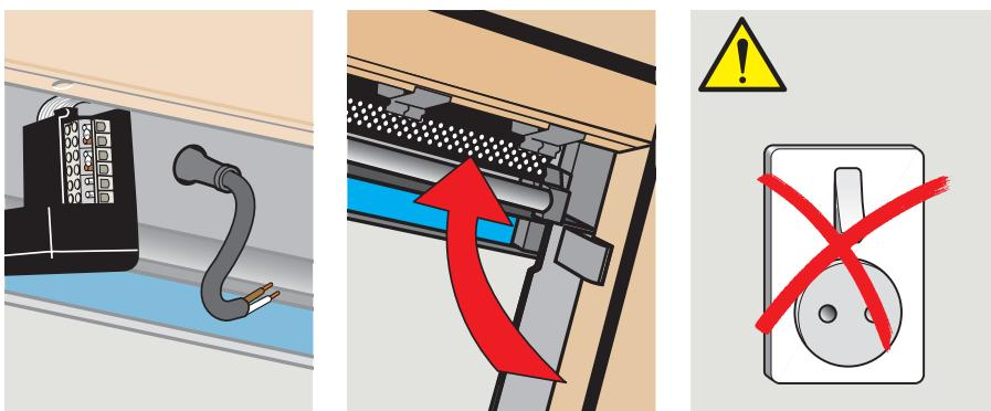
**ENGLISH:** Connect the cable to terminal block or connection box. For connection to control unit, refer to instructions for control unit/remote control. If the window was fitted with a connection box, refit box.
